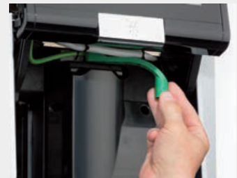
Swing the green handle left to right to re-lock hoppers
