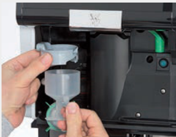
Separate top of bowl and remove hose
