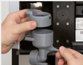
Separate top of bowl and remove hose
